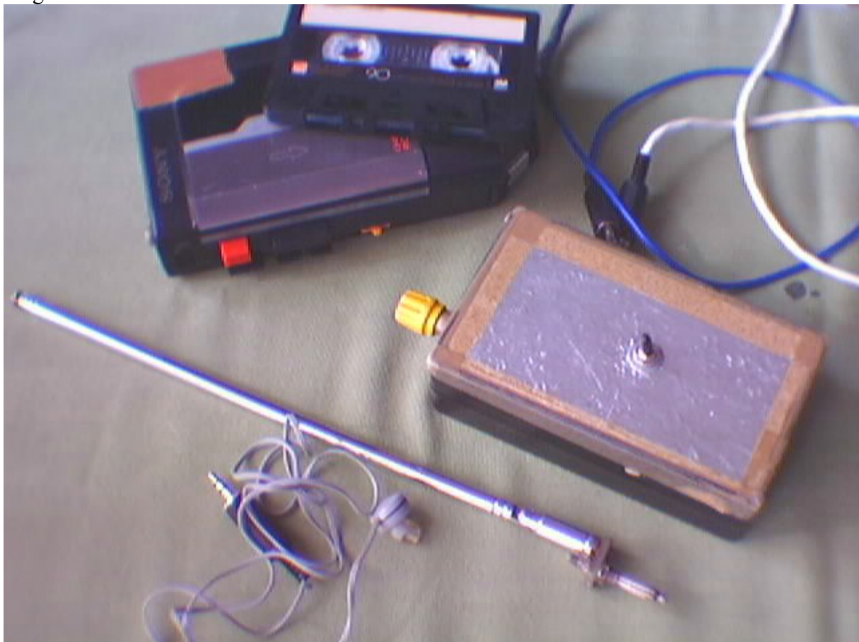
My equipment: VLF receiver, whip antenna, earphones, cassette tape recorder, audio cable
