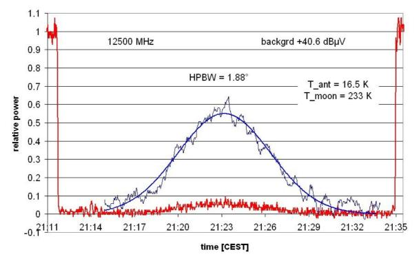
This demonstrates that a good background subtraction is of crucial importance for the interpretation of weak signals, such as from the moon. This affects the antenna temperature and hence the deduced source temperature: The lunar temperature came down from 233 K to 135 K. One must emphasize that this large change in the absolute value is mainly due to the
