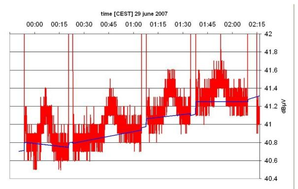
Reducing the data with the above backgrounds and using the analytical fit to the calibration data, and smoothing the reduced data with a box-car average of about 50 points gave these results:
