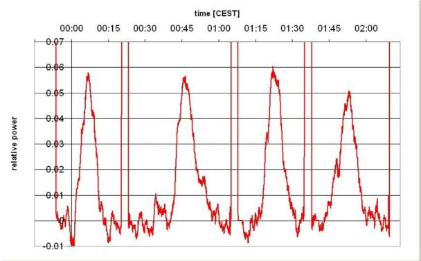
The four scans show a satisfactory background subtraction and that the peaks have the same values. We must except the fourth scan, which suffered from either the arrival of the cloud cover or a non-central passage through the antenna lobe.
