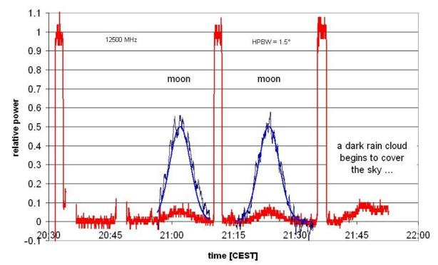
These successive scans were helpful in confirming that establishing that we do observe the moon, but we also could identify the failure of a third scan with a dark rain cloud passing over that region of the sky. In the first two scans, the sky contained a thin veil of clouds which apparently did not affect the observations, giving a very constant background signal. The rain cloud's signal is comparable with the lunar signal, and even exceeds it.
