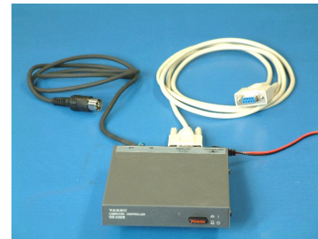
PC interface for motor controller Yaesu GS-232B
