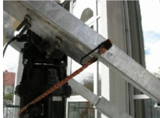
Fig. 11. Rubber Band anchored to Dish Support Frame [Assembly Manual p. 14]
