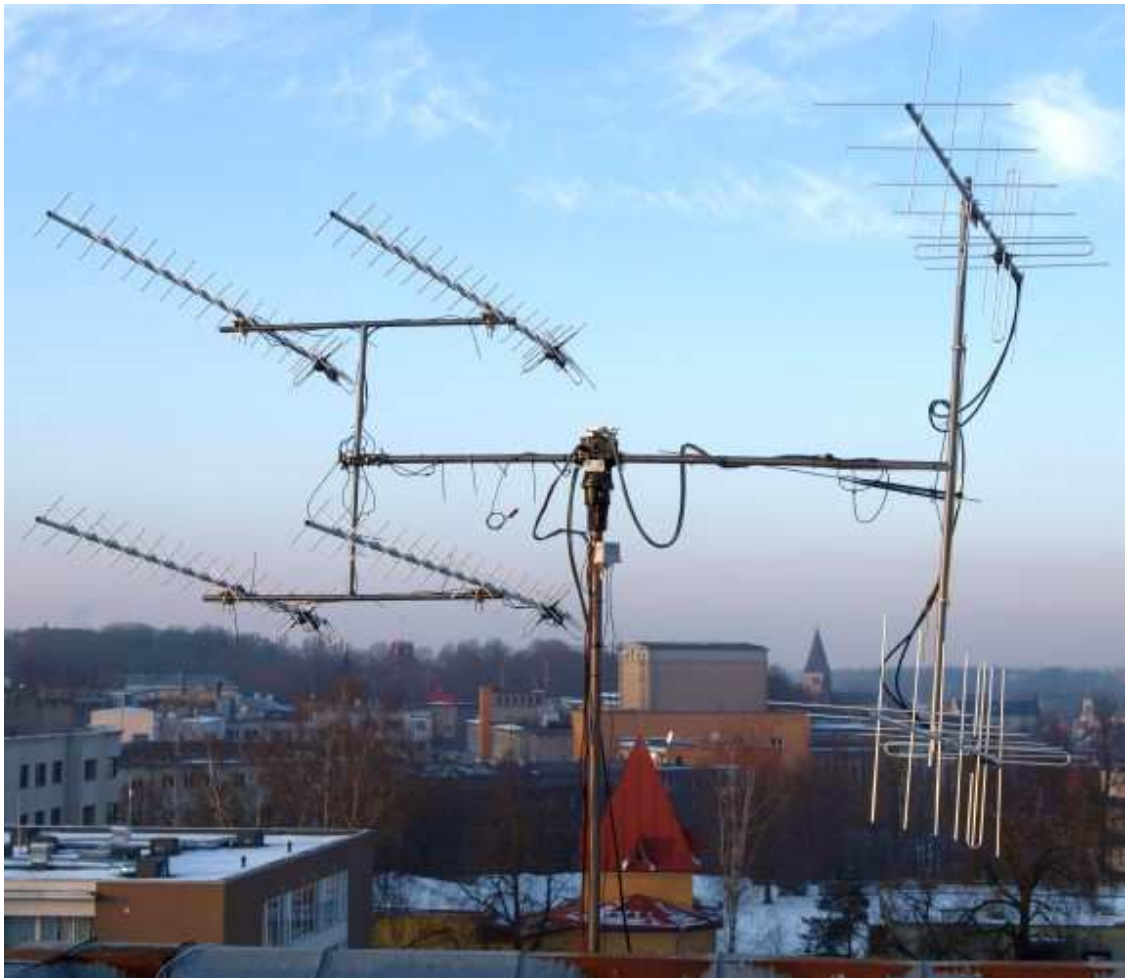
Figure 5.1 The Tartu University Ground Station antenna system mounted on the top of Physics Department building (Estcube Team, 2008).
