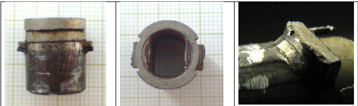
Fig.6 The coupling ring (original state) viewed from the side (left) and the top (centre Fig.8 ). The lower part of a tooth shows heavy wear, while the top side is untouched (right Fig.9 ).
