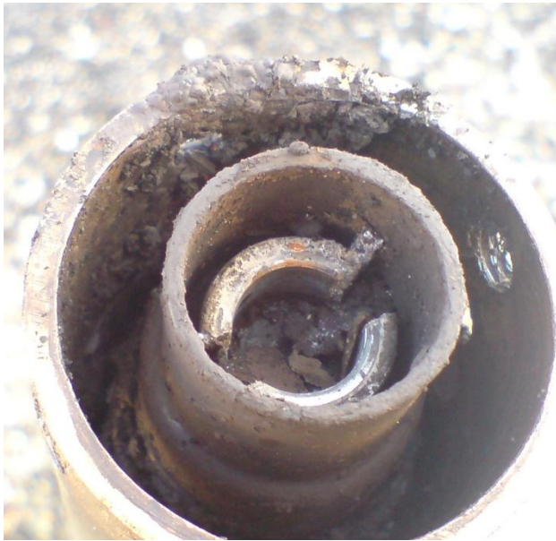
Fig.2 At the bottom end of the linear actuator tube a substantial amount of black residue was found in Jan.13, which appears to be mixture of the original lubricant, the applied oil, and perhaps metal rubbings.
