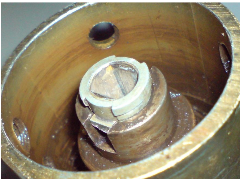
Fig.11 The reduced coupling ring now engages fully with the threaded rod's slots.
