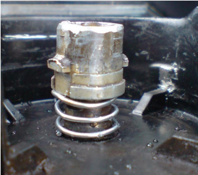
Fig.14 The reduced coupling ring is held up by a small compression spring.
