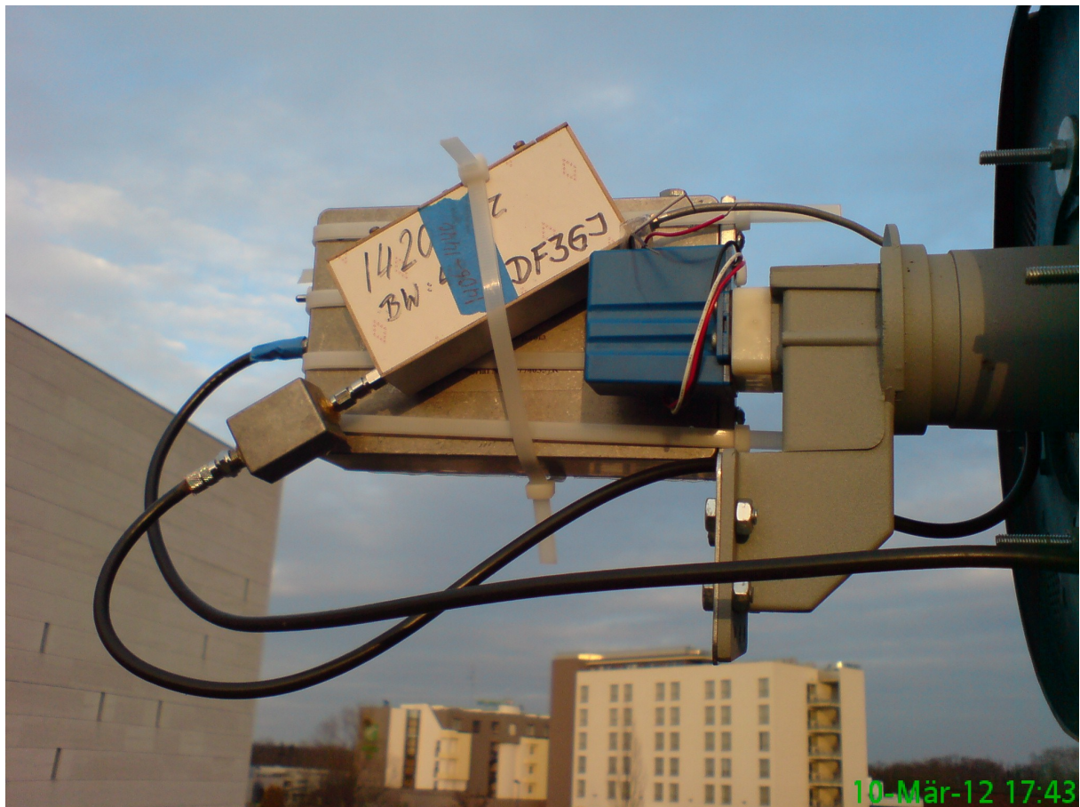
Fig.4 The improved focal assembly: in the foreground are the small preamplifier and the narrow band filter, in the background the large receiver box. The blue box and the waveguide structure at right are not used.
