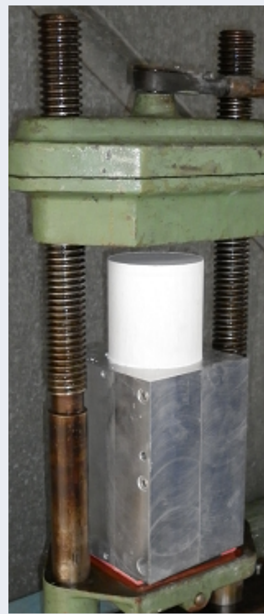
Figure 2: Press with dust agglomerate
