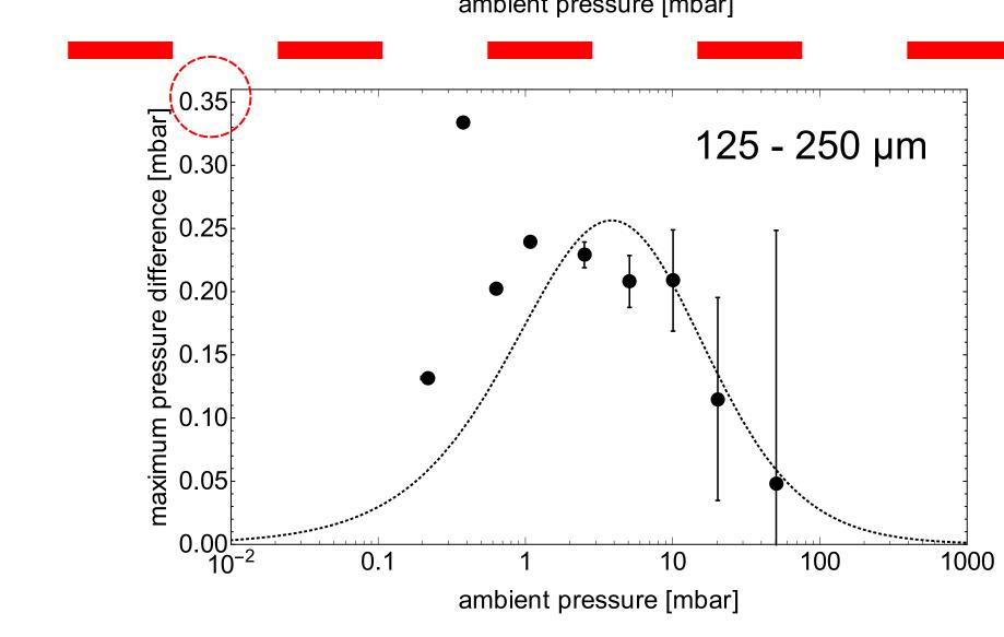
The three figures on the left side show the maximum pressure difference  $\Delta p_{\text{max}}$ reached through the Knudsen compressor for spherical glass particles with different size distributions and JSC Mars 1A dust. The black dotted lines represent the fit function Eq. (1) with  $T_{\text{hot}}$  as free fit parameter. To get a more realistic fit function an additional particle size analysis was made for every dust sample. Two size distributions are shown below.
