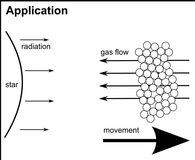
A porous body in a protoplanetary disc is heated on one side by the radiation of the star, which induced the Knudsen engine gas flow through its pores and pushes it in a farther orbit.
