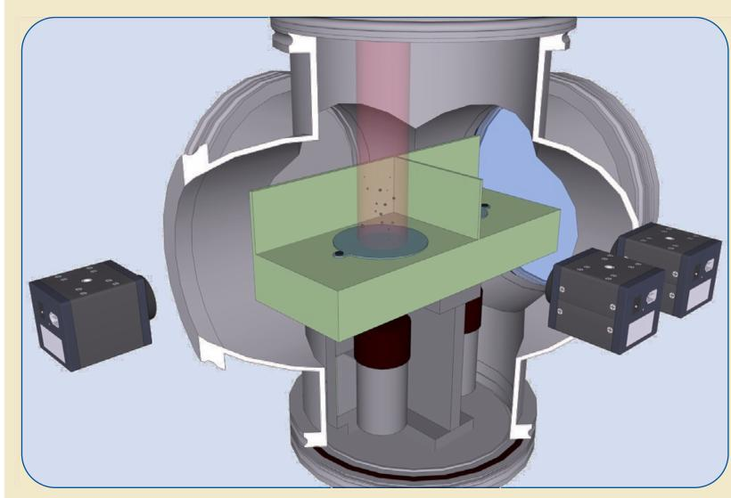
Sketch of the setup: A 7 cm dust bed is il*luminated by an IR laser (955 nm). The* Laser Spot is widened to achieve a power density of 20 kW/m<sup>2</sup> with a beam diameter of 3.4 cm at the surface of the basaltic dust sample. Only one camera was used for this study.
