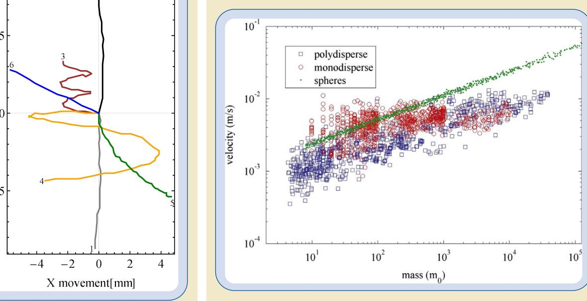
Drift velocity versus mass, normalized to the mass and velocity of a  $r = 1 \mu m$  sphere ( $m_0$ ) =  $1.3 \cdot 10^{-14} \text{ kg}, v_0 = 1.1 \text{ mm s}^{-1}$ ). (Monodisperse  $r = 1.7 \ \mu m$ , Polydisperse r =
