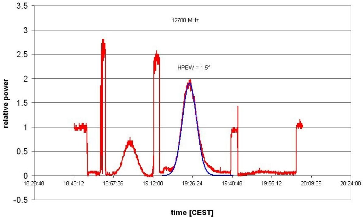
Finally, it was found that the setting of the background level is rather crucial for the shape of the subtracted lunar profile. The figure below show the fit of background and calibration levels during the lunar scans:
