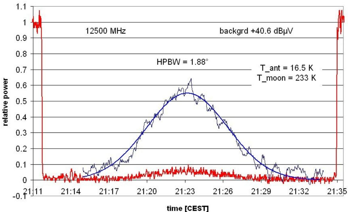
This demonstrates that a good background subtraction is of crucial importance for the interpretation of weak signals, such as from the moon. This affects the antenna temperature and hence the deduced source temperature: The lunar temperature came down from 233 K to 135 K. One must emphasize that this large change in the absolute value is mainly due to the
