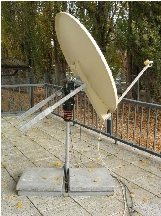
Figure 2 Outdoor and Indoor unit of the school radio telescope
