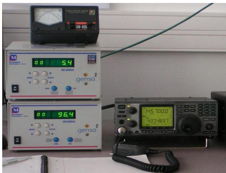
Figure 1-2 The ISU Ground Station's control equipment
