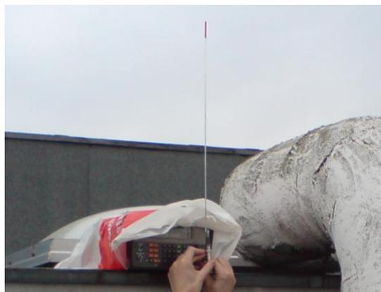
Figure 4-8 Signal generator and its antenna
