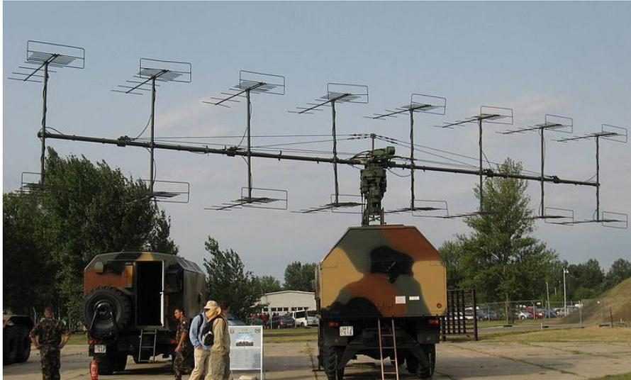
Figure 1-4 The stacked antenna of P-18M radar [reference 6]
