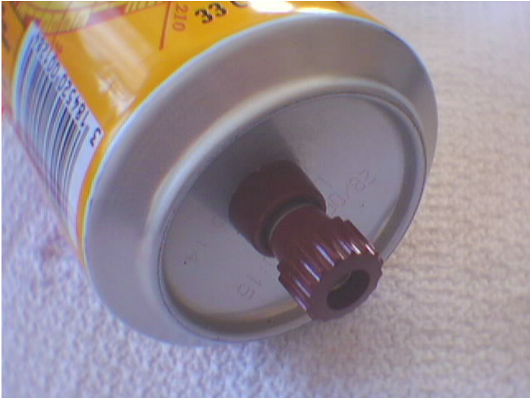
The antenna terminal of a beer can VLF receiver
