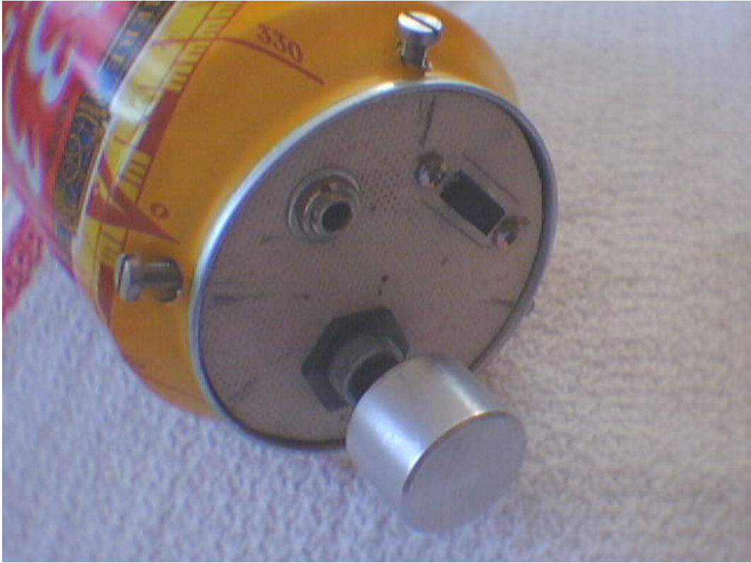
The lid of the beer can is replaced by a printed circuit board which carries the controls
