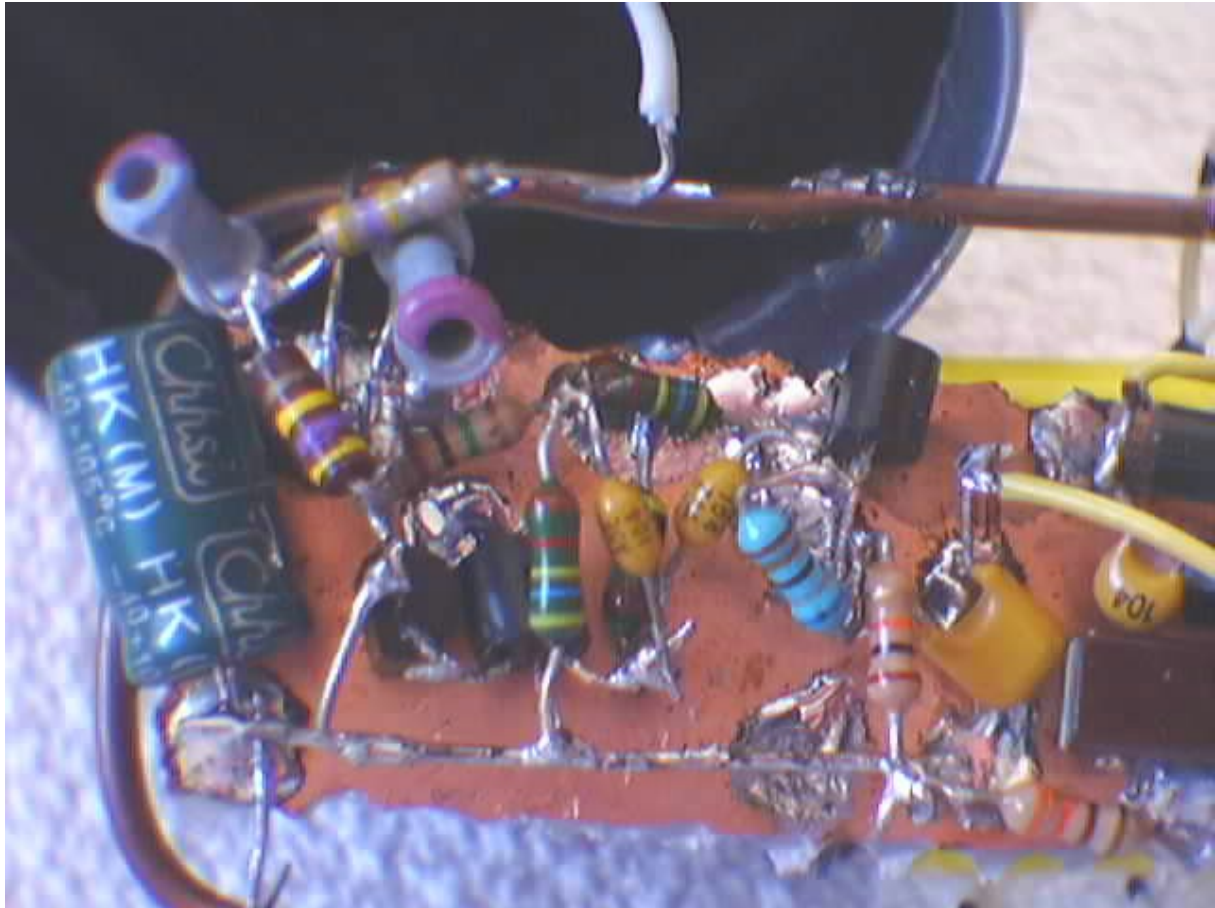
Input filter and impedance conversion stage built in ‘free-style’ using an empty printed circuit board as ground plane
